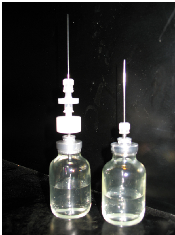
Fig. 4. MDI with the traditional injection apparatus (left), and modified injection coupler (right).
